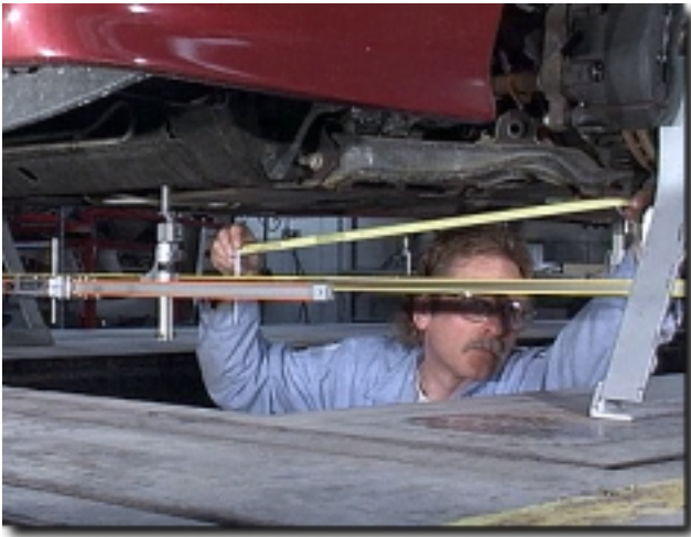
D-2 Tram gauges are measuring tools used to make quick checks during damage analysis.
