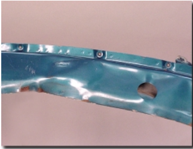
C-2 These coined surfaces are used to align panels on the vehicle structure.
