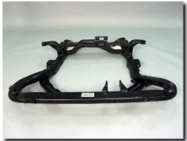
C-3 Hydroforming creates seamless, one-piece structure, such as this engine cradle, from a steel sheet or tube.
