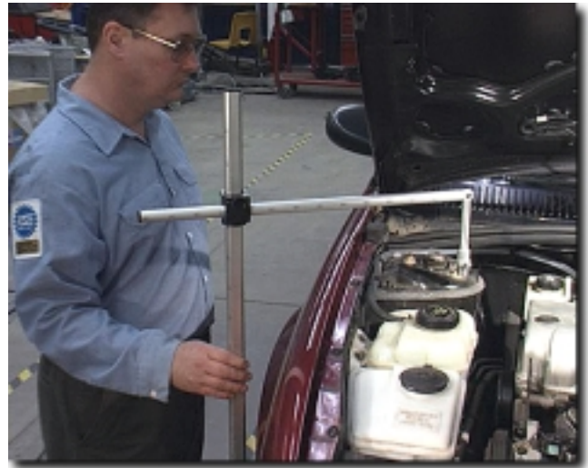
D-4 Repair tolerance should not be more than 3 mm for the entire vehicle.
